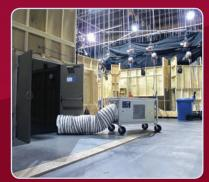
Sound stages can be difficult or expensive to adequately heat. Using this electric furnace enabled this production to provide heat where it was needed most.
