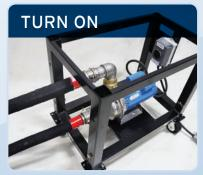
A single phase, 30 amp, 208 volt circuit energizes these units, and a simple on/off switch controls when you want them running.
