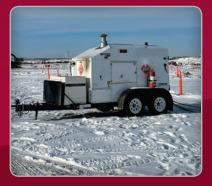
The HGT400 can thaw up to 6000 square feet using the on-board hose reel. With additional hose, it can thaw up to 8000 square feet.
