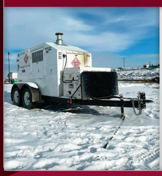
This portable central heat plant is easily towed and set up quickly. Its 7 kW generator enables complete standalone operation, making it essential for thawing frozen ground before excavation, curing concrete, or providing emergency heat when your building's boiler or hot water system fails.
